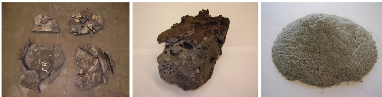
Fig. 7. Metal alloy (left), slag (middle) and flue dust (right) produced in technical-scale test.
