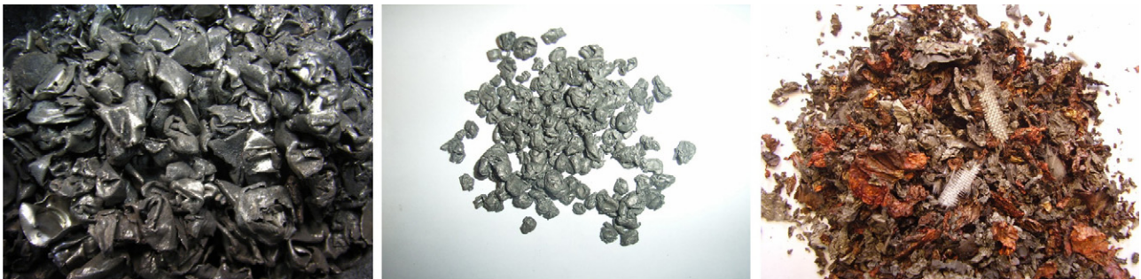
Fig. 3. Metal containing material fractions after crushing and material separation (from left to right: iron-nickel fraction, aluminium fraction, electrode foil fraction).
